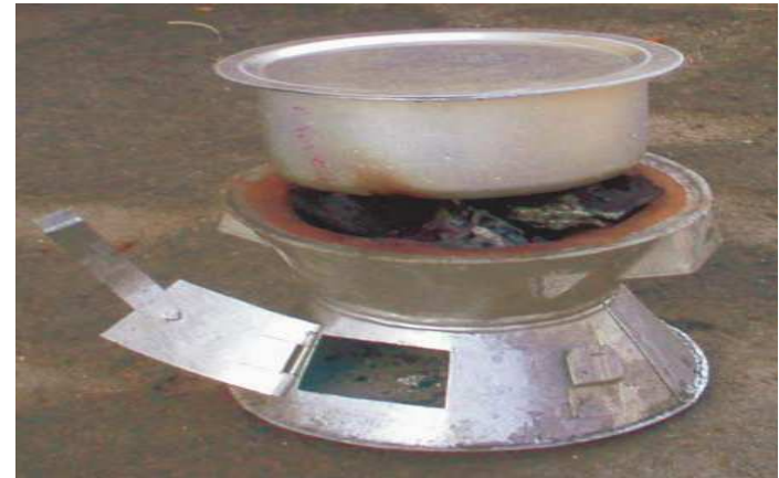
“Laketch Charcoal Saving Stove” in 25-35% efficiency
